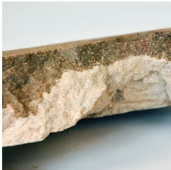
STOPGAP SRS Penetrates a weak friable surface to reinforce prior to applying further treatments
