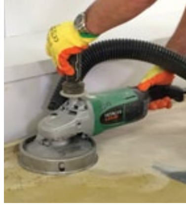
Hand held grinders can easily remove adhesive residue or surface treatments
